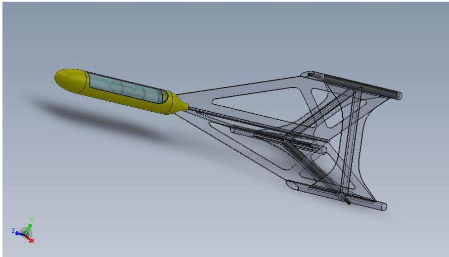
Fig.25: Mechanical support for the magnetic sensors and housing for the electronics of the 2D gradiometer designed to be towed by an AUV. Notice that the geometry of the gradiometer can be adapted provided that the arrangement of the individual vector sensors allows for the acquisition of the magnetic gradient tensor.
