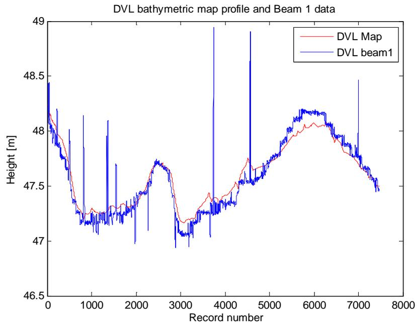
Fig.15-a: Profile of altitudes (expressed in WGS84 datum) measured by DVL beam#1 during the tests with the Medusa ASV along the path shown in Fig.14, superimposed on the corresponding profile of the reference map.
