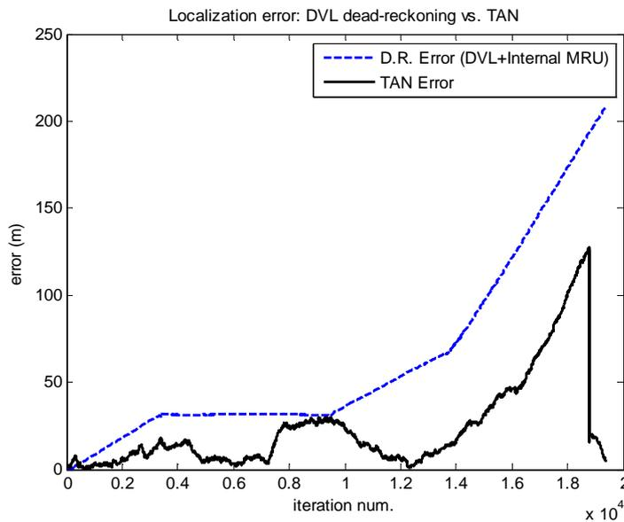
Fig.18: Absolute value of the localization error obtained with TAN and Dead-reckoning performed with the DVL data.
