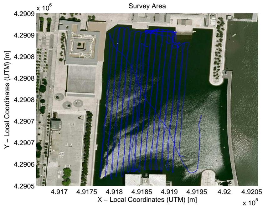
Fig.2: Trajectories used for bathymetric data acquisition with the Doppler at the test site.
