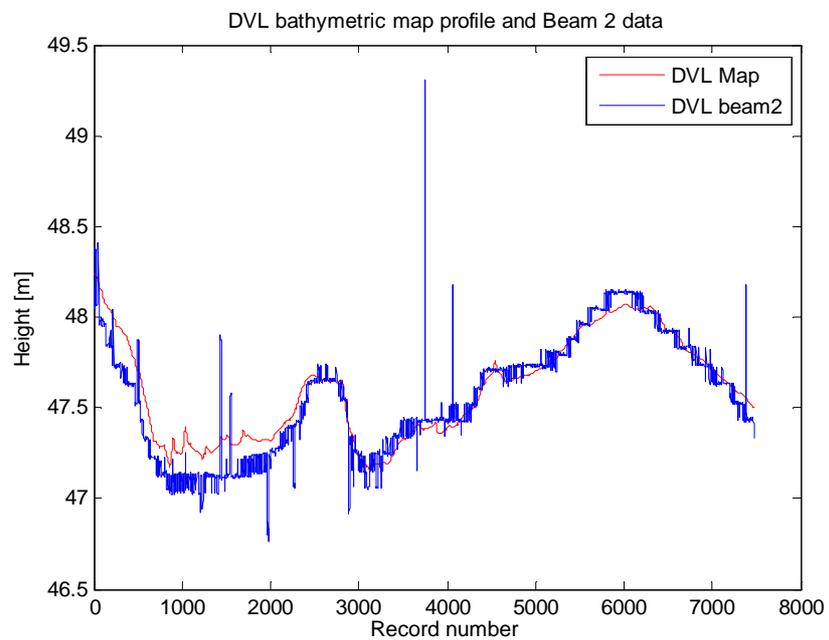
Fig.15-b: Profile of altitudes (expressed in WGS84 datum) measured by DVL beam#2 during the tests with the Medusa ASV along the path shown in Fig.14, superimposed on the corresponding profile of the reference map.
