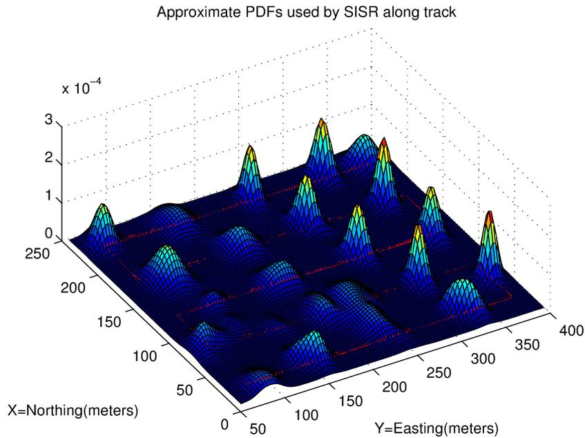
Fig.9-a: Probability density functions (PDFs) used by the standard Particle Filter SISR. Compare with the following figure and notice the biased estimates and much larger uncertainty of the standard filter SISR shown here that is caused mainly by terrain symmetries and areas of flat terrain to which the PPF proves to be very robust.
