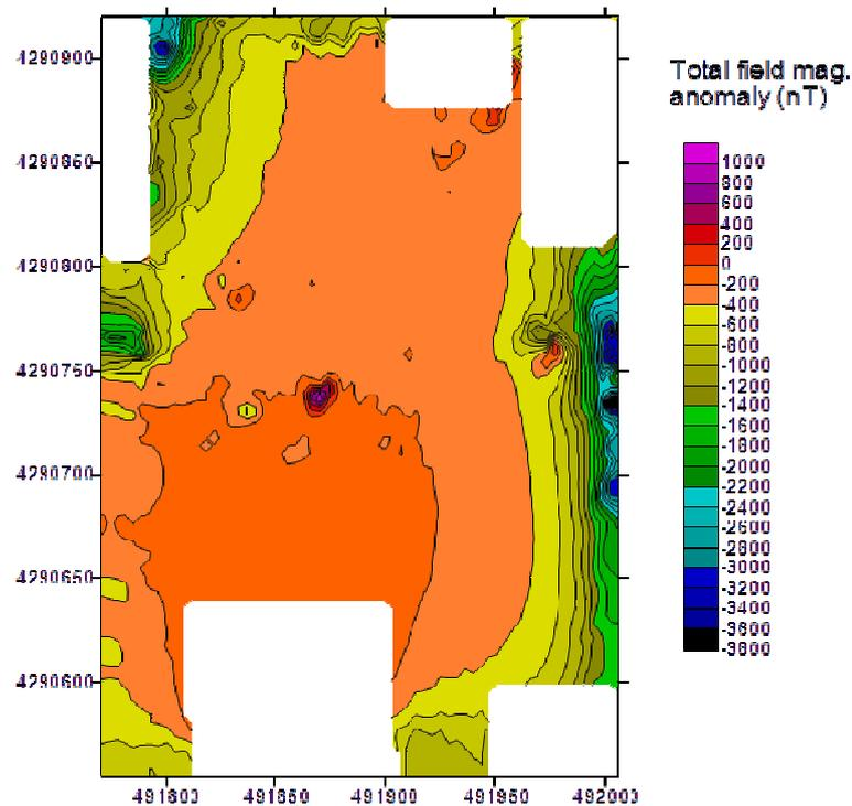
Fig.6: Magnetic anomaly map of the trial site. Some areas are blanked in the map since they are not useful in terms of geophysical navigation and their high amplitude prevents showing enough detail in the areas of interest.
