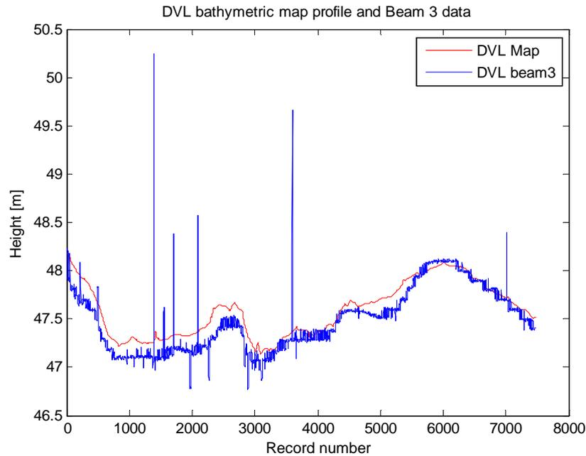
Fig.15-c: Profile of altitudes (expressed in WGS84 datum) measured by DVL beam#3 during the tests with the Medusa ASV along the path shown in Fig.14, superimposed on the corresponding profile of the reference map.
