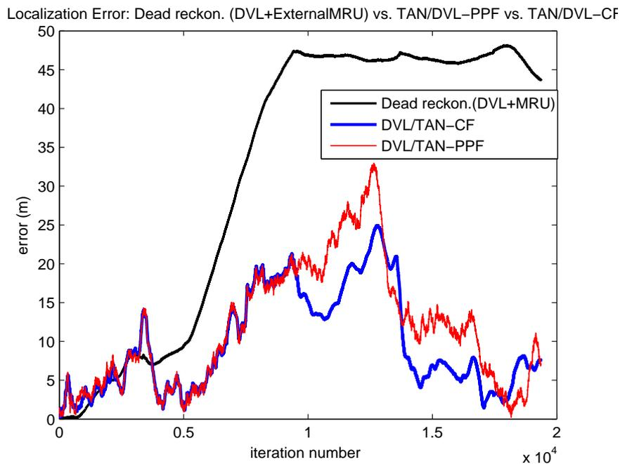
Fig.22: Absolute value of the localization errors obtained by conventional DVL dead-reckoning compared with those obtained with the new geophysical navigation methods.
