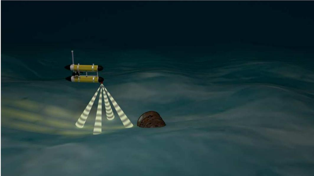
Fig.12: Terrain Aided Navigation using a Doppler velocity logger.
