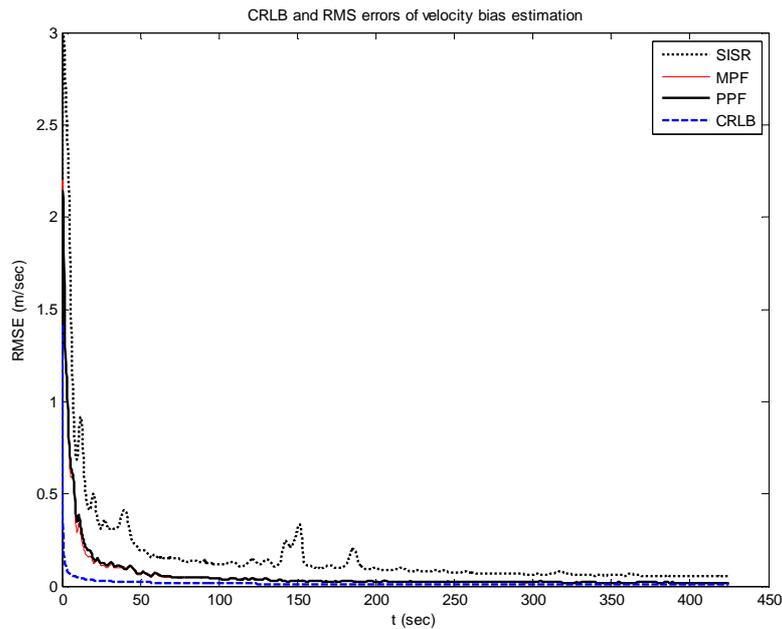
Fig.8: Velocity (bottom) estimation error obtained by the new (MPF and PPF) and the prior (SISR) navigation methods compared with the theoretical lower bound (CRLB) obtained in simulations with real data.
