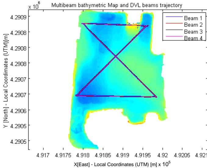
Fig.14: Trajectories of the experimental trials executed by the ASV *Medusa* at the test site, superimposed on the bathymetric. Notice that each trajectory comprises four simultaneous records of altitudes measured by the four beams of the DVL. The results obtained with this trajectory are illustrated in the following figures.
