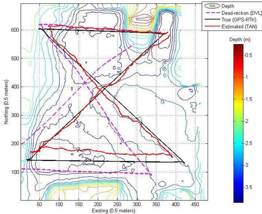
Fig.19: True trajectory, dead-reckoning (DVL + External IMU), and TAN estimated trajectory.
