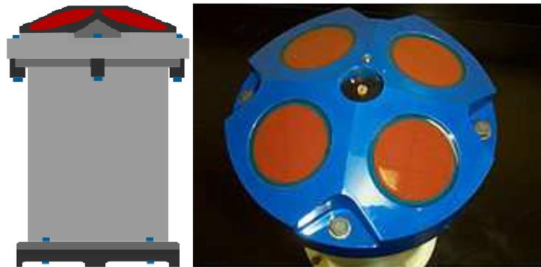
Fig.10: Side view diagram (left) and head view (right) of the Doppler velocity logger (DVL) used in the tests of geophysical navigation. Notice the arrangement of the four sonar transducers which allow for the acquisition of 4 simultaneous range measurements.
