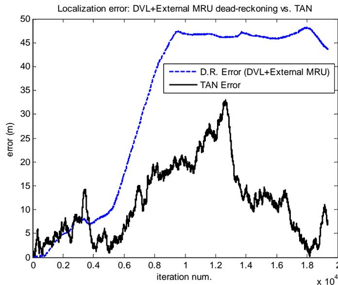
Fig.20: Absolute value of the localization error obtained with TAN and Dead-reckoning performed with the DVL and the external MRU data.
