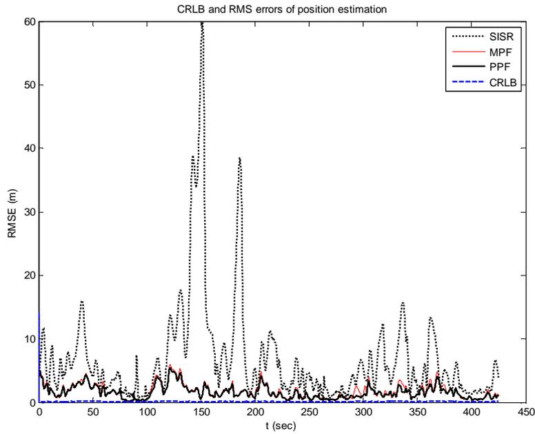
Fig.7: Position estimation error obtained by the new (MPF and PPF) and the prior (SISR) navigation methods compared with the theoretical lower bound (CRLB) obtained in simulations with real data.
