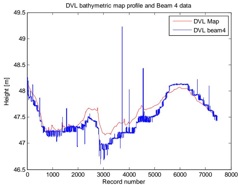
Fig.15-d: Profile of altitudes (expressed in WGS84 datum) measured by DVL beam#4 during the tests with the Medusa ASV along the path shown in Fig.14, superimposed on the corresponding profile of the reference map.
