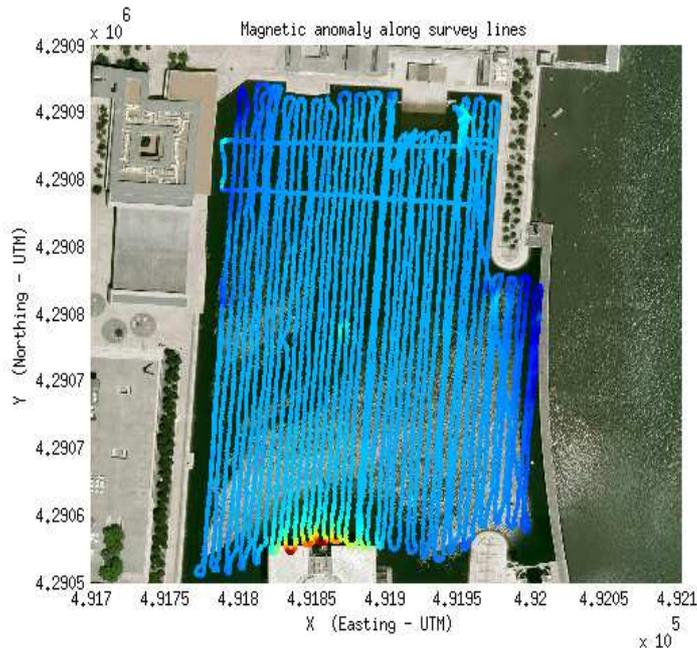
Fig.5: Magnetic survey performed with a scalar magnetometer at the test site and preliminary profiles of the magnetic anomaly observed. A second, identical scalar magnetometer was used as a base-station to allow for correction of diurnal variations of the Earth's magnetic field.
