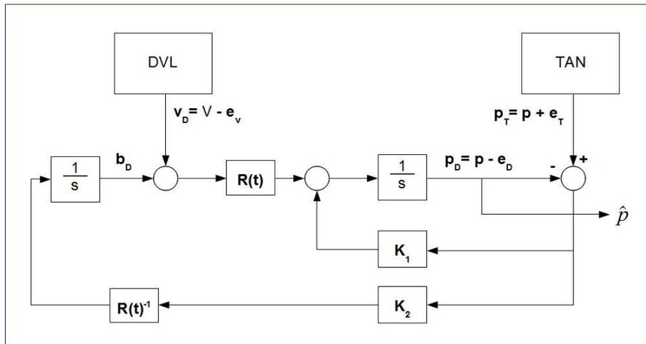
Fig.21: Structure of the complementary filter used to integrate the TAN output with DVL dead-reckoning.
