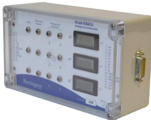
Fig.26: The Analog Correction Unit (ACU) supplied by Bartington Instruments, Ltd. This unit was used to acquire the gradient measurements during system calibration.
