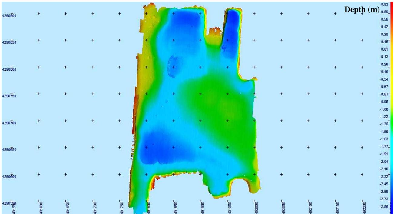
Fig.4: High-resolution bathymetric map of the test site acquired with a multi-beam sonar (UTM Northing and Easting coordinates in meters).
