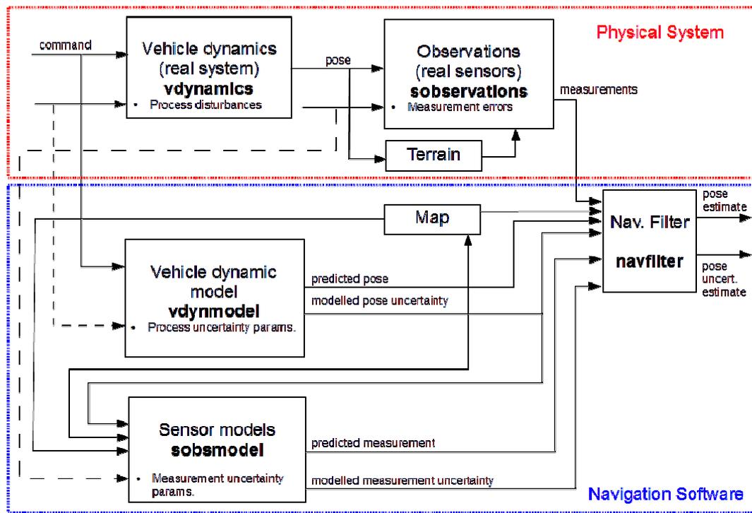
Fig.13: Architecture of the Geophysical Navigation software used in simulations, ready for integration in the AUV.
