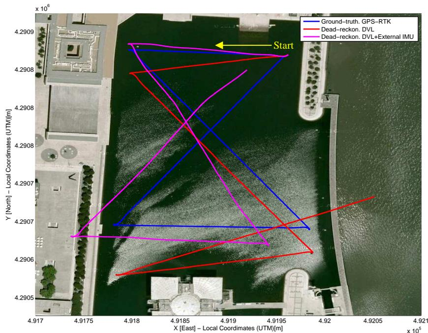
Fig.16: True trajectory (blue) and dead-reckoning estimates obtained with different motion sensor units; the yellow arrow indicates the direction of vehicle motion at the point of departure.
