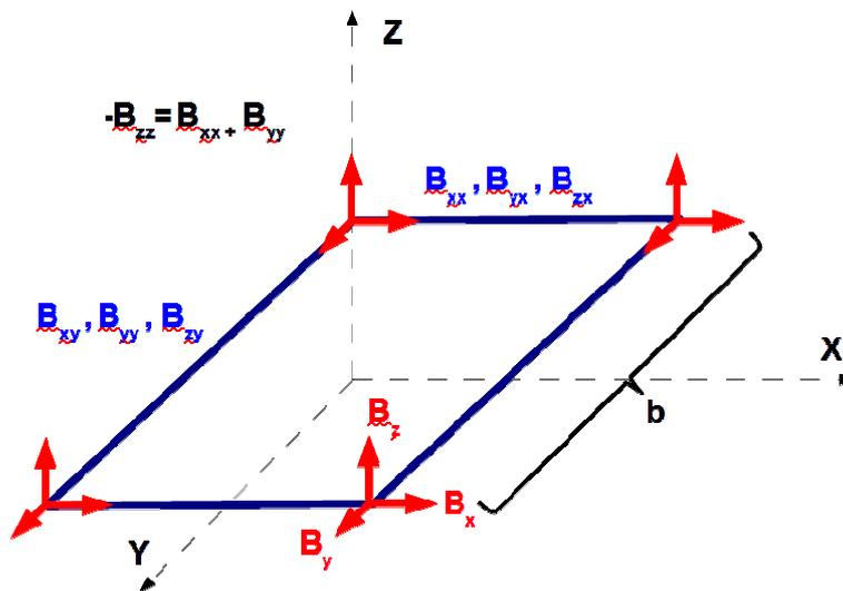
Fig.24: Schematic arrangement of the 3-axial magnetic sensors in the bi-dimensional magnetic gradiometer. The variables  $B_i$  denote the components of the magnetic field vector and  $B_{ij}$  denote their spatial derivatives corresponding to the components of the magnetic gradient tensor.  $B_i$  and  $B_{ij}$  are measured directly by the gradiometer but some components are computed from the measured quantities;  $b$  is the gradiometer baseline.
