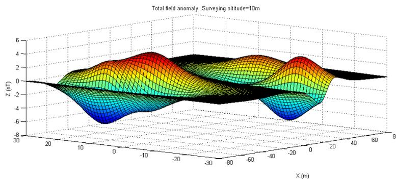
Fig.27: Multi-pole magnetic anomaly modeled by the software package developed in Matlab for magnetic-based geophysical navigation.
